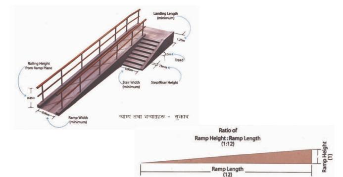
The ramps represent on of the main equipments for universal accessibility. Ramps are the slope to enable the persons with mobility limitation to access the infrastructure.
